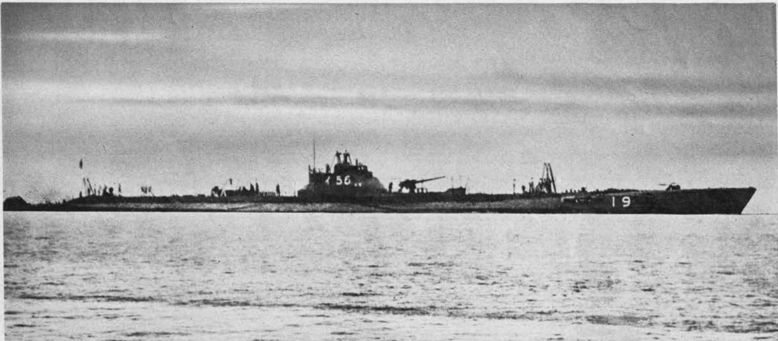
STANDARD JAPANESE FLEET SUBMARINE RESEMBLES THIS I-153 DESIGN. FORWARD BULGE ON CONNING TOWER, VERTICAL RUDDER ARE PROMINENT
